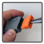
Step 1: Remove orange wedge by pulling it straight out using appropriate tool.
