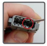
Step 2: Remove contacts with a gentle pull while at the same time releasing the locking finger with a screwdriver.
