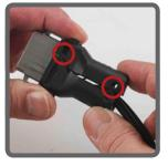
Step 3: Close the connector back shell properly until a CLICK is heard. Avoid squeezing wires.
