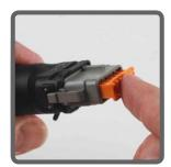
Step 4: Once all necessary contacts are in place, insert orange wedge until it snaps into place.
