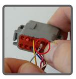
Step 3: Hold the seal in place with your finger, while pulling out the contact.
