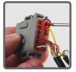
Step 1: Use appropriate tool to push contact straight into the connector grommet until a CLICK is felt.
