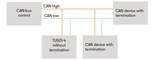
**NB!** When the unit is stub connected, the wire length must be minimized to avoid CAN-bus noise and error ratio.
