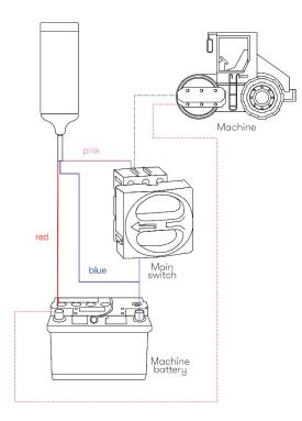
In case the main breaker is on the negative wire (ground wire from the machine battery), the inputs may register a voltage level and start counting operating hours.
