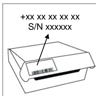
GSM number and unit serial number is located on the box. Label can be peeled off and saved for later use.
